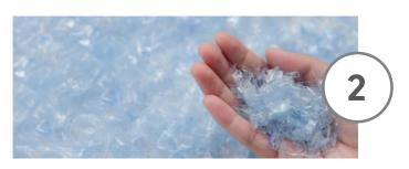
The discarded soda and drinking bottles are cleaned and cut into flakes before being melted and extruded into fibers of natural white color.
