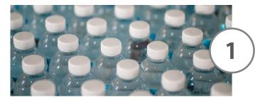
Acoufelt acoustic panels are made from postconsumer plastic beverage bottles out of landfills and oceans. Every square foot of panel contains the regenerated fibers made from approximately 6.6 (20oz) recycled bottles.
